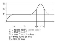
(2) Soldering iron method Tip temperature: 350 to 400°C 662 to 752°F Wattage: 30 to 60 W Soldering time: within 3 s (3) Others Check mounting conditions before using other soldering methods (DWS, VPS, hot-air, hot plate, laser, pulse heater, etc.) • The temperature profile indicates the temperature of the soldered terminal on the surface of the PC board. The ambient temperature may increase excessively. Check the temperature under mounting
