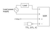
6. Self Sustaining Circuit Using SSR
