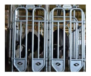
Has the cow finished eating? Then she leaves the feeding station through a gate at the front, that opens after the signal from an infrared sensor to the control system. Not every sensor is suitable for this, says Bart. "Just think of the environment: it's dirty quickly, so the sensor has to cope with that. Also, the sensor should not distinguish between color and stain pattern, so that the gate opens for each cow."
